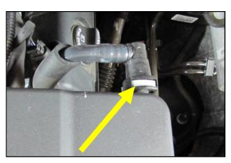
2. The quick connects for the valve cover breathers are removed by depressing the grey locking tab in the fitting and sliding them away.
